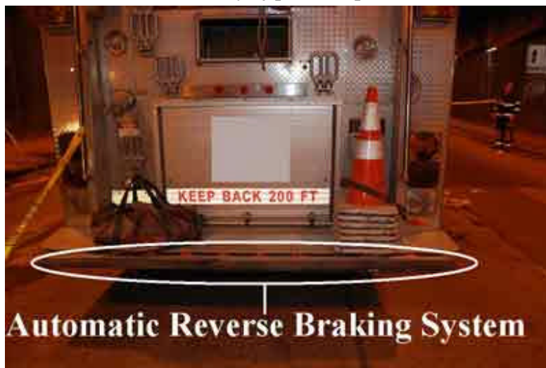
Photo 2. This reverse braking system is attached to the rear bumper of the apparatus and is designed to actuate the rear brakes when pressure is applied to the rubber
