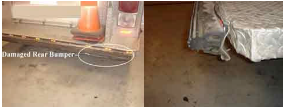
Photos 3 and 4. Pictures show damage to rear bumper and rubber sensor. (Photo courtesy of PEOSH.)
